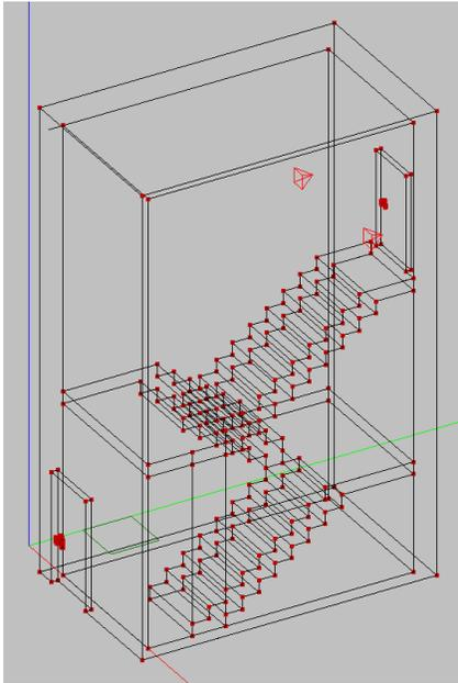
Figure 2: EASE Model of Staircase
