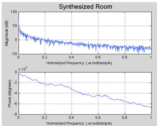
Figure 14: FFT of sim. impulse response
