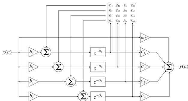
Fig. 1. Length-4 Feedback Delay Network
